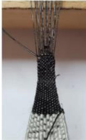
Weaving with carbon nanotube thread consisting of ~300 microfibers produced by over winding on the take-up reel.
